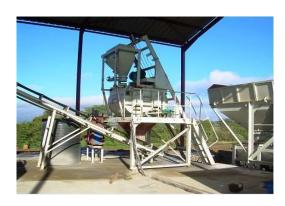
**2. Mixer---** the dosed materials will be lifted by the skip elevator to the mixer for mixing.
