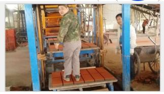
**3. Block Machine--**The mixed materials will be transferred to the block machine, After vibration and compaction of the mould, The fresh blocks will be produced.
